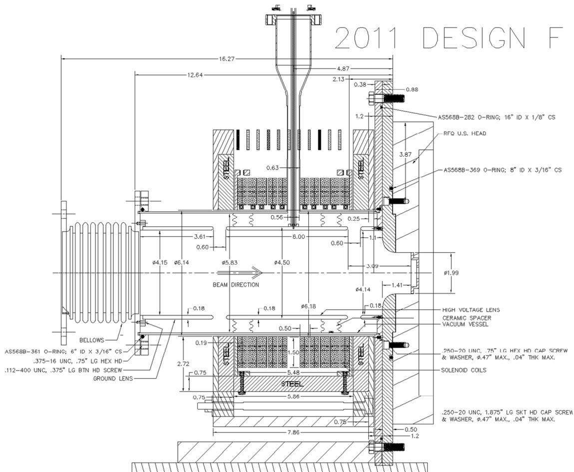
Figure 1: Design of the New Solenoid- and Einzel lens system for the front of the RFQ. The Distance between RFQ and solenoid was decrease by 1.08 inches.
