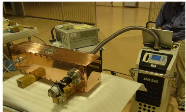
Figure 3: New 201.25 MHz copper buncher for the MEBT with Q (loaded) 3500.
