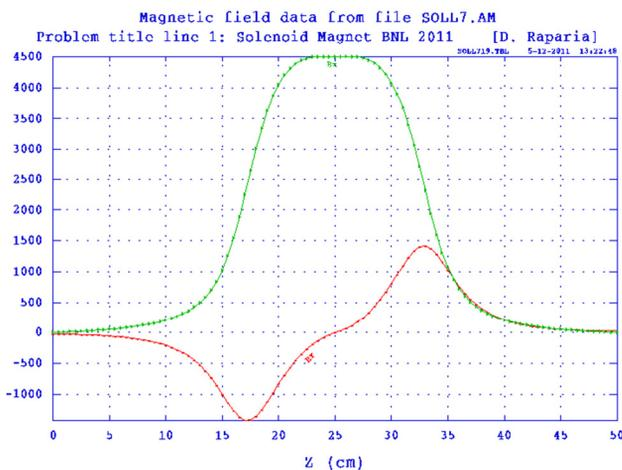
Figure 2: Magnetic field component Br and Bz along the length of the solenoid at 5 cm radius.
