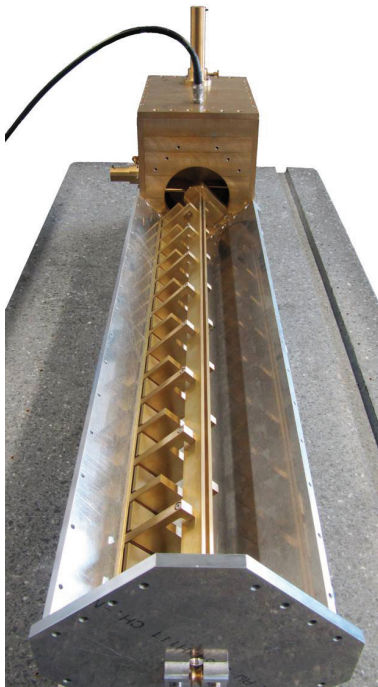
Figure 1: Coupled 1:2 RFD-DTL model for investigation of the coupling between two different accelerator structures. The RF-dipole (RFD)-model shows a capacity load per meter which is equivalent to the RFQ structure.
