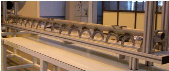
Figure 8. Laser welded prototype cavity support system
