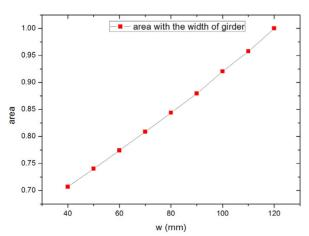
Figure 5: The surface of CH cavity with the width of girder.
