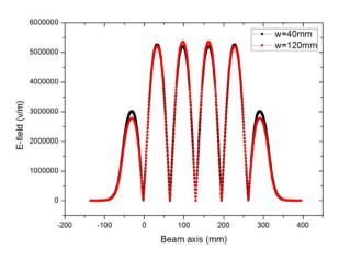
Figure 6: Field distribution of CH cavity with the different width of girder.
