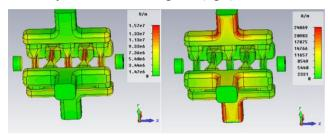
Figure 3: The electric field of use undercut CH cavity (left) and the magnet field of use undercut CH cavity.
