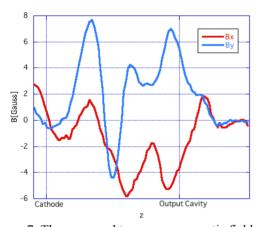
Figure 7: The measured transverse magnetic fields.
