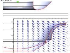
Figure 9: The calculated magnetic field in the cathode area
