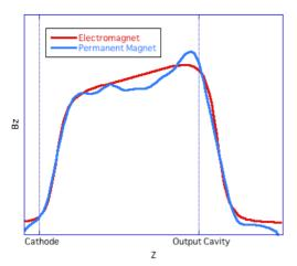
Figure 5: The longitudinal magnetic fields.
