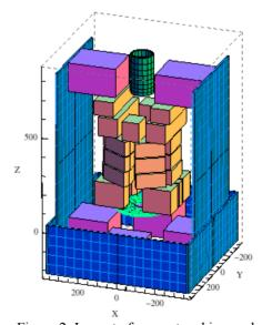
Figure 2: Layout of magnet and iron yoke.
