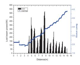
Figure 4: The lost beam power distribution when the first cavity breaks down at 10mA.
