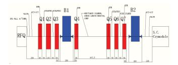
Figure 5: Layout of beam diagnostics in MEBT.
