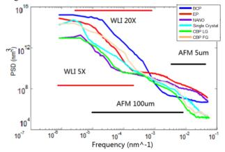
Figure 2: Joint 1D PSD models from AFM/WLI are shown and the characterization frequency domains are indicated.
