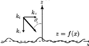
Figure 1: A plane wave incident impinging on a rough surface with incident angle  $\theta_i$ .
