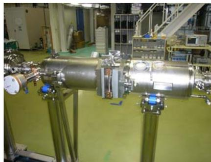
Figure 6: Attachment of a slide-jack and a piezo tuner.
