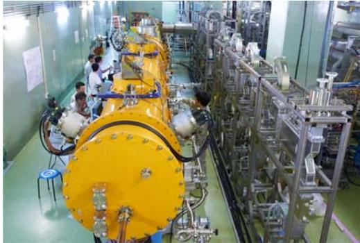
Figure 8: S1-Global cryomodule in the STF tunnel.
