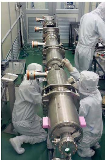
Figure 5: String assembly of four Tesla-like cavities.
