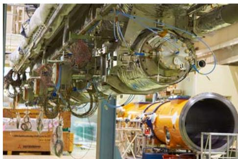
Figure 7: String cavities hung on a He gas return pipe.
