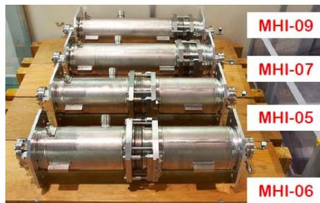
Figure 2: Four Tesla-like cavities for S1-Global.
