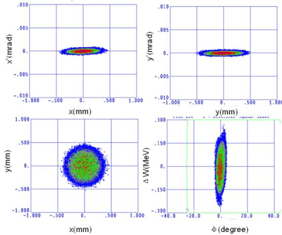
Figure 2: Phase-space distribution at the exit of the DTL.
