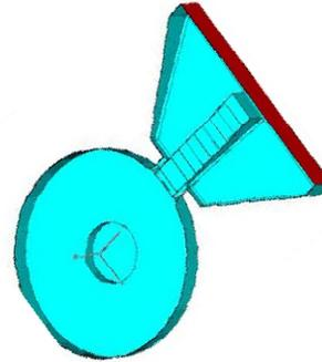
Figure 3: 3D simulation of the waveguide coupler.
