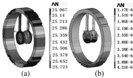
Figure 5: Temperature distribution (a) and thermal expansion (b) of the DTL tank wall.
