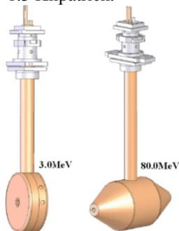
Figure 6: CSNS DTL drift tubes at 3.0 and 80.0MeV.
