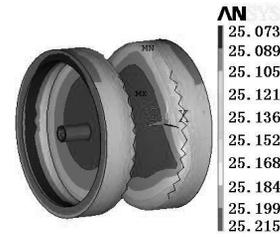
Figure 7: Temperature distribution on the tube surface.
