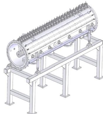
Figure 4: The design model of Alvarez-type DTL cavity.
