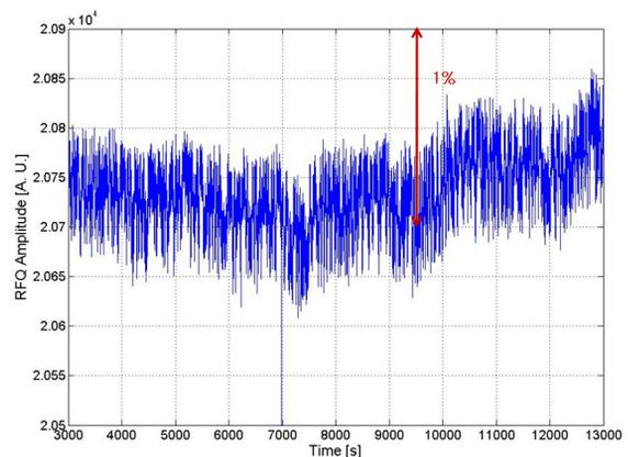
Figure 5: RF amplitude during 20MeV linac operation.
