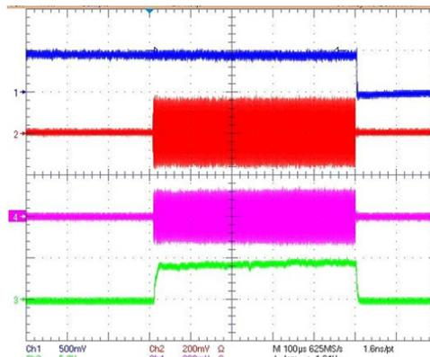
Figure 7: LEPT, RFQ and DTL output beam pulse for 500us operation. (Ch 1: LEBT current, Ch 2: RFQ current, Ch 3: DTL current, Ch 4: DTL current (Faraday cup)).
