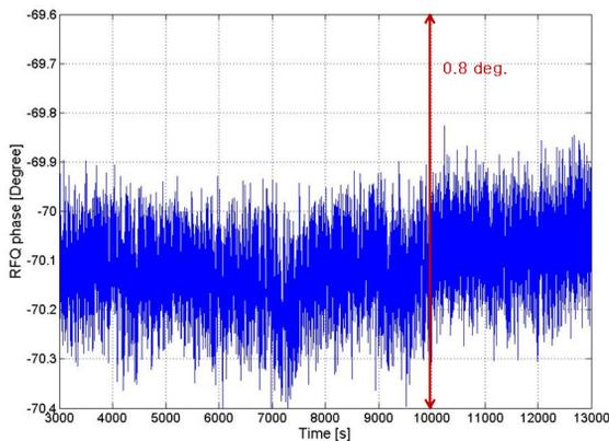
Figure 6: RF phase during 20MeV linac operation.
