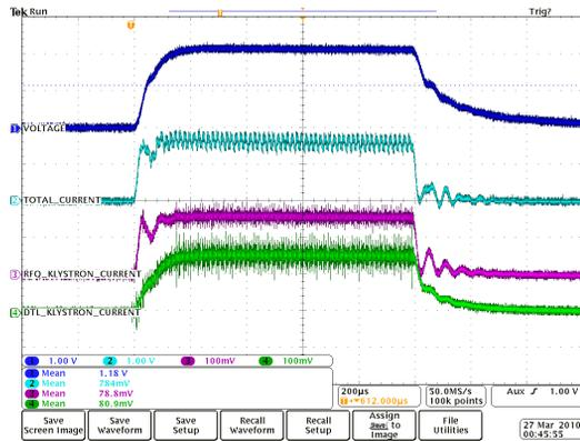
Figure 2: Modulator voltage and current pulse profile.
