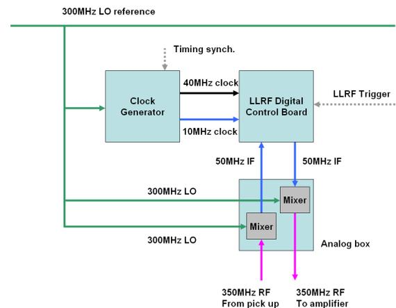
Figure 4: Block diagram of the modified LLRF system.
