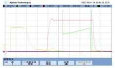
Figure 7: Pulsed discharge current (red) of 50 A with a pulse width of 800  $\mu$ s and the extraction beam current (green) about 300 mA with a pulse width of 520  $\mu$ s.
