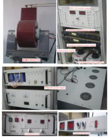
Figure 3: Main power supplies for ion source.
