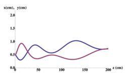
Figure 7: Beam envelope in the DWA with a periodic quadrupole focusing channel provided by deformed HGIs.
