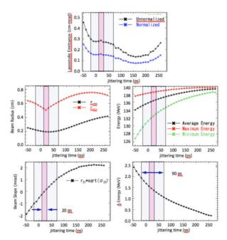
Figure 4: Proton bunch's Lapostoll emittance, beam radius, beam slope, energy and energy variation at the DWA exit versus injector timing jitter.
