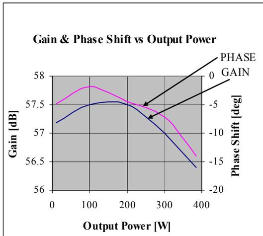
Figure 5: Gain and phase measurement of the solid state driver amplifier.
