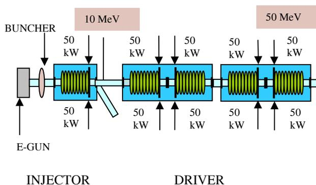
Figure 1: Basic layout of the E-linac.
