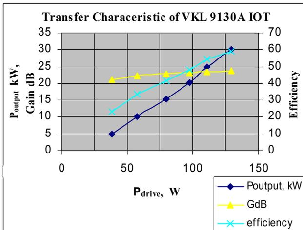
Figure 4: RF measurement of the IOT up to 30 kW output power.
