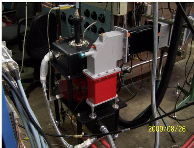
Figure 3: Photo of the 30 kW IOT in a test set up at the factory.
