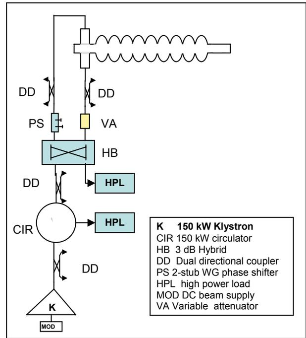
Figure 6: Basic scheme of 150 kW klystron rf system.
