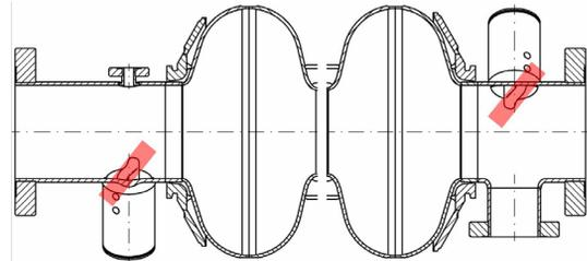
Figure 5: "in line" position of the DESY HOM-couplers.
