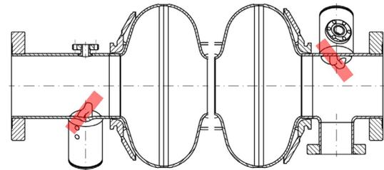
Figure 6: "mirrored" position of the DESY HOM-couplers.
