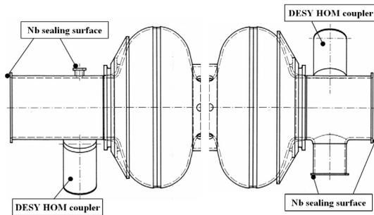
Figure 3: Base design of the first 1.3GHz TESLA cavity.
