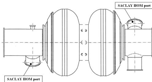
Figure 4: Cavity with SACLAY HOM coupler ports.
