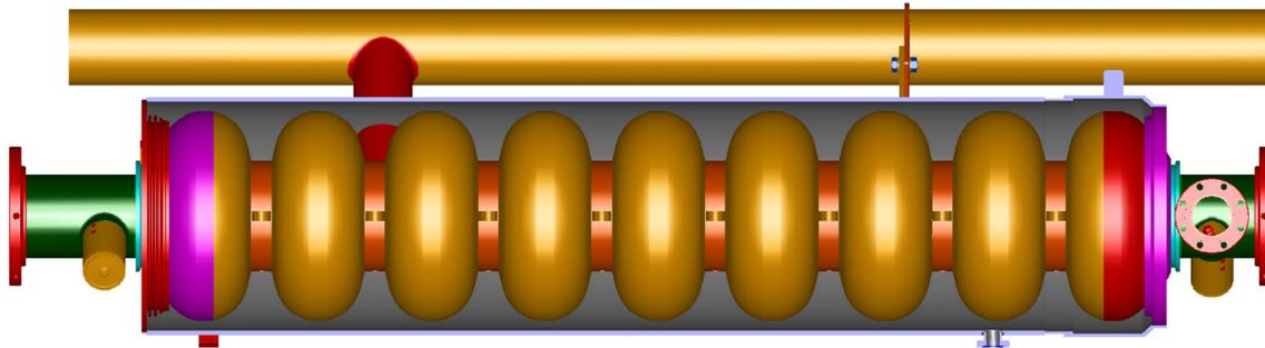
Figure 7: Picture of the 3D-Modell of the 1.3GHz cavity in helium tank for the European XFEL.
