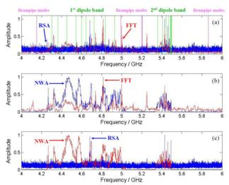
Figure 5: Comparison of spectra taken by Scope (after FFT), RSA (after concatenation) of C1H1 and NWA (transmission measurement without beam-excitation). The vertical lines indicate the simulation results. All spectra are normalized to the highest amplitude in frequency span of 4 GHz to 6 GHz.
