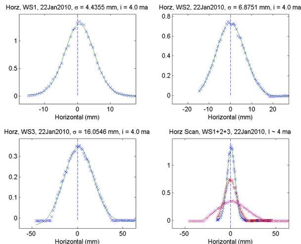
Figure 3: Transverse beam profile measurements from three wire scanners after RFQ. Solid lines are Gaussian fits to measured data points. Lower right plot is an overlay of all three scanner profiles.
