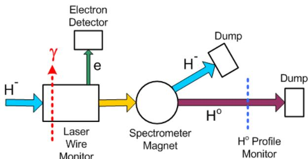
Figure 6: A block-diagram of a proposed laser transverse emittance monitor.
