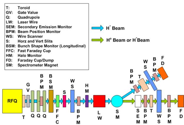
Figure 5: Proposed layout of HINS beam diagnostic R&D beamline.
