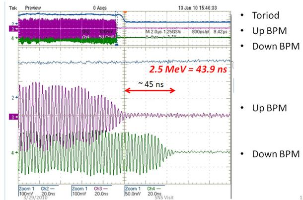
Figure 4: A measure of the RFQ beam energy derived from time-of-flight between two BPMs.
