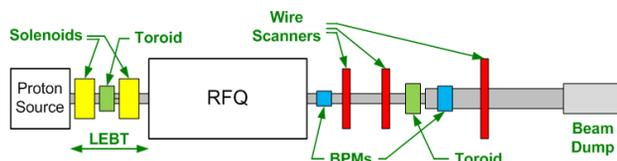
Figure 1: Block diagram of the beamline configuration used for the initial RFQ beam measurements.
