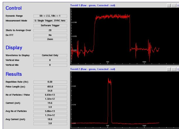
Figure 2: HINS LEPT (top) and RFQ output (bottom) beam currents. The RFQ RF power was limited to 50  $\mu$ s to minimize heating issues.
