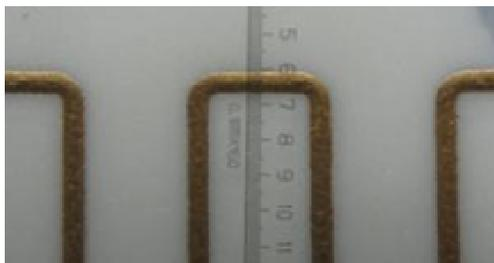
Figure 6: strip width reductions at corners.
