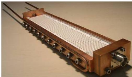
Figure 1: Electrode prototype on its support.
