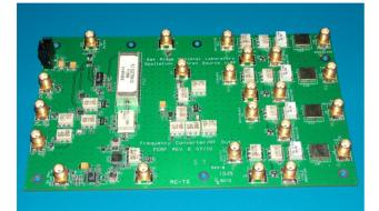
Figure 3: Frequency Conversion RF Board
