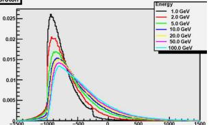
Figure 7: Hadronic shower energy deposition as a function of longitudinal position (in mm) and incident proton energy, from a calorimetry study by A. Para [5].
