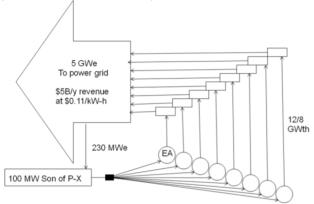
Figure 6: Schematic of a large power station that is driven by an SRF proton linac that could be developed using the proposed Fermilab Project-X. The 100 MW beam is distributed to 8 thorium-burning Energy Amplifiers (EA) as in Figure 4 above. Each EA feeds a steam turbine to provide power to the national grid.
