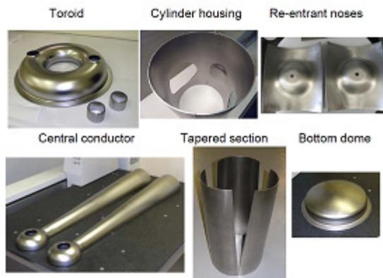
Figure 6: Various cavity niobium parts as die forming complete.
