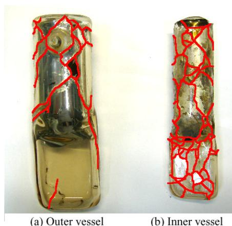
Figure 9: Restoration photographs by jointing of fragments of dewar flask exploded.
