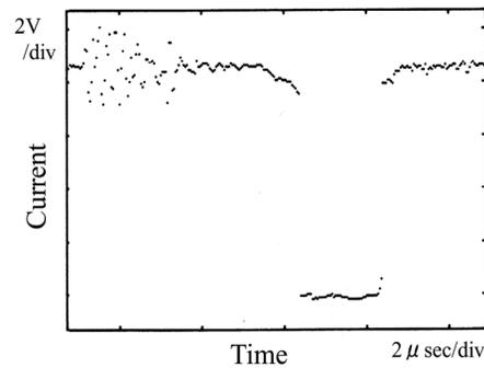
Figure 1: Pulse shape of the electron linear accelerator.
