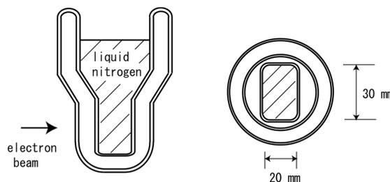
Figure 5: Dewar flask for liquid nitrogen using in the explosion experiment.
