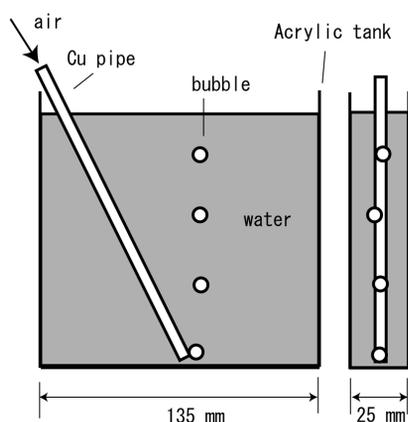
Figure 3: Moving object for testing the electron strobography system.
