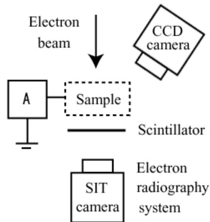
Figure 2: Electron radiography system.
