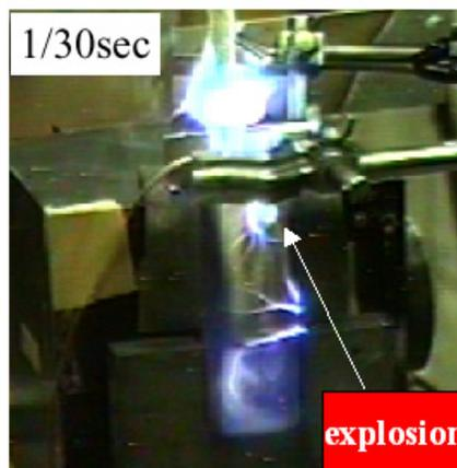
Figure 7: One flame image at the moment of explosion.
