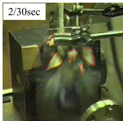
Figure 8: One flame image after the explosion. Fragments of broken dewar are enclosed by red line.
