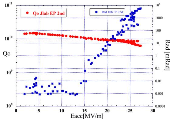
Figure 6: VT after 2<sup>nd</sup> EP at Jlab.
