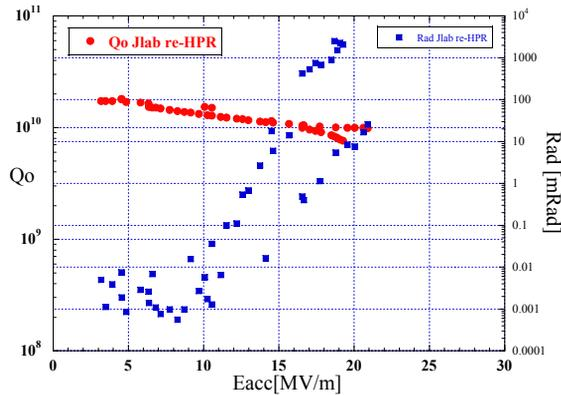
Figure 5: VT after re-HPR at Jlab
