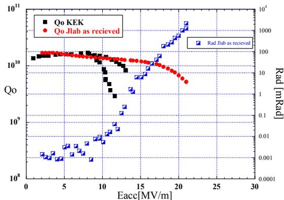
Figure 3: VT at KEK and as received at Jlab.
