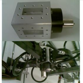
Figure 3: WR284 waveguide switch (above) and switch assembly in situ (below).
