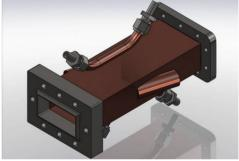
Figure 7: Design for a new arc detector viewport.
