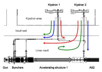
Figure 2: The new waveguide configuration.
