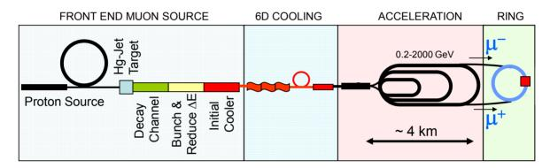
Figure 4: Neutrino Factory [2,3] and Muon Collider [1] schematics.
