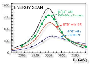
Figure 2: Comparison of collision energy spreads for 3 TeV  $e^+e^-$  and  $\mu^+\mu^-$  colliders. Top black curve is before radiative effects are included. Green curve shows muon collider energy spread including initial state radiation (ISR) and beamsstrahlung (BS), Red curve shows the impact of ISR on an  $e^+e^-$  collider, and the bottom blue curve shows the combined effects of ISR+BS on an  $e^+e^-$  collider
