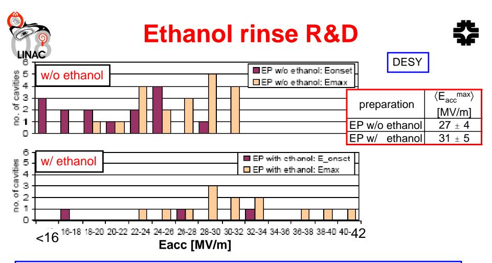
Ethanol rinse immediately following final EP to remove sulfur particles
