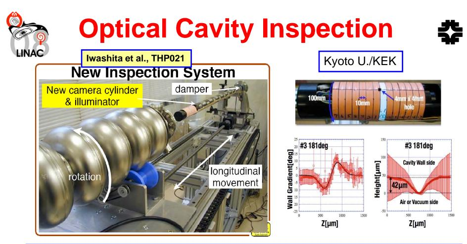
Illumination by electroluminescent strips which can be turned off/on individually: shadows can be analyzed for 3D defect mapping (pit vs. bump) [bump is shown]
