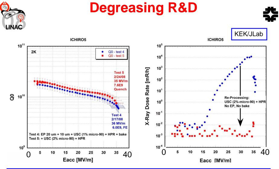
One example: KEK 9-cell Ichiro-shape cavity tested at JLab
