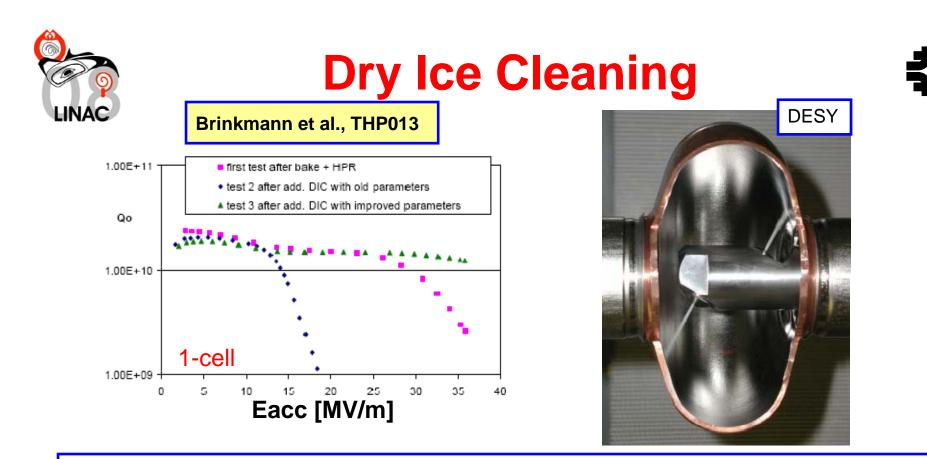
Rapid cooling embrittles contaminating particles
