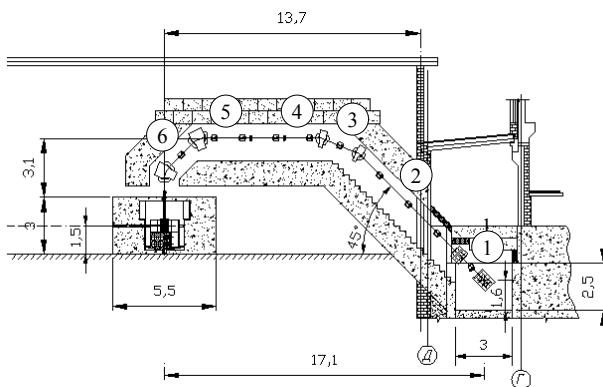
Figure 2. Layout of the transportation channel from the linear accelerator to the sub-critical assembly. Vertical plane.
