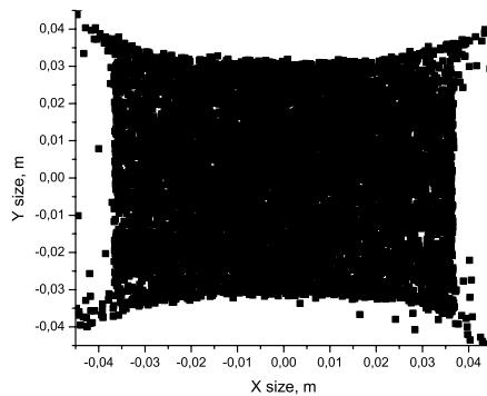
Figure 3. Transversal coordinate distribution of the driving electron beam at the target of the neutron source.
