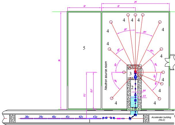
Figure 1. Layout of the Neutron Source Location: 1 – linear accelerator; 2 – electron beam transport channel; 3 – sub-critical assembly; 4 – neutron channels; 5 – express laboratories building.
