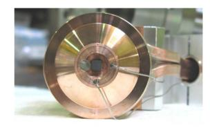
Figure 2: Positron production target assembly with a hole.
