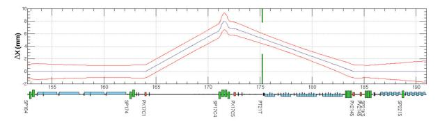
Figure 1: Target bypass orbit and beam-line component layout around the positron production target.
