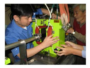
Figure 3: Pulse steering magnet for target bypass orbit
