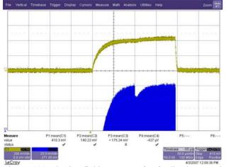
Figure 4(a): Cavity field response for feedback control. (upper: Forward RF power, lower: Cavity field)
