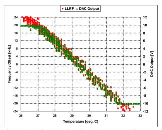
Figure 6: DAC output based on the measured frequency offset from the resonance.
