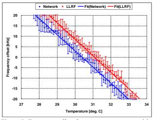
Figure 5: Frequency offset from resonance measured by network analyzer and LLRF system.
