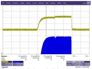
Figure 4(b): Feedback control with Feed-forward. (upper: Forward RF power, lower: Cavity field)
