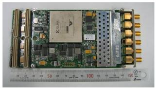
Figure 1: ICS-572B PMC Board.
