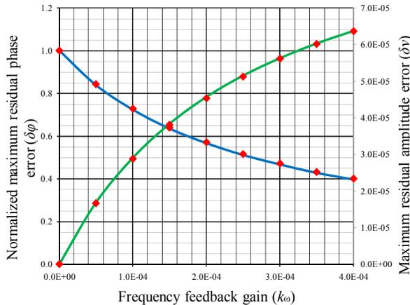
Figure 3: Maximum amplitude (green) and phase (blue) residual errors as a function of  $k_\omega$ . Simulation results are in red.
