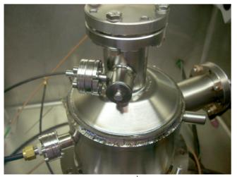
Figure 7: Close-up view of 3<sup>rd</sup> harmonic cavity with helium vessel after TIG welding is complete.
