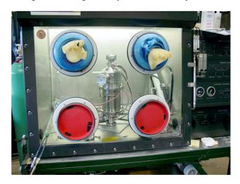
Figure 5: Glove box with cavity installed for TIG welding. Note the cables for monitoring the frequency spectrum of the cavity, and the lines for passing argon through the cavity and helium vessel during welding.
