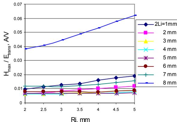
Figure 5: Iris radius  $\times H_{max}/E_{trans}$  for different iris lengths.
