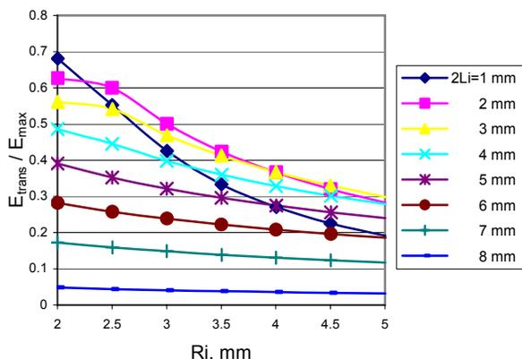
Figure 4: Iris radius  $\times E_{trans}/E_{max}$  for different iris lengths.
