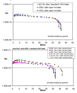
Figure 5 a+b: Comparison of open Ar-bake with standard UHV-bake after final short BCP (top); typical Q(E)-curves after final short BCP and UHV-bake (bottom).
