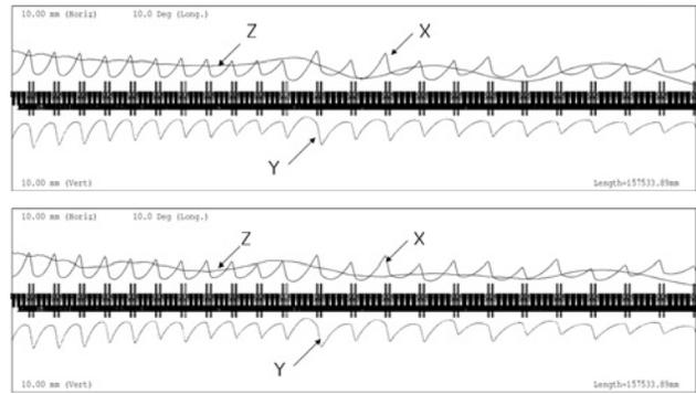
Figure 7: Trace3D envelope profiles for the smooth focusing optics (upper plot) and those for the constant phase optics (lower plot).
