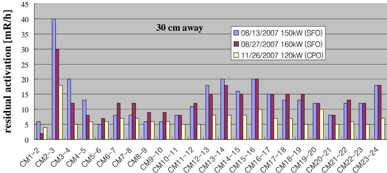
Figure 4: Plots of the residual machine activation 30 away after the beam operation for three different run periods. The 150 kW (08/13/2007) run and the 160 kW (08/27/2007) run used the “Smooth Focusing Optics (SFO)”, while 120 kW (11/26/2007) run the “Constant Phase Optics (CPO)”. CM1-2 means that between the cryo-module 1 and 2.
