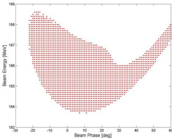
Figure 6: Plot of the longitudinal acceptance when the phase of all cavities are set to the design values without any matching.
