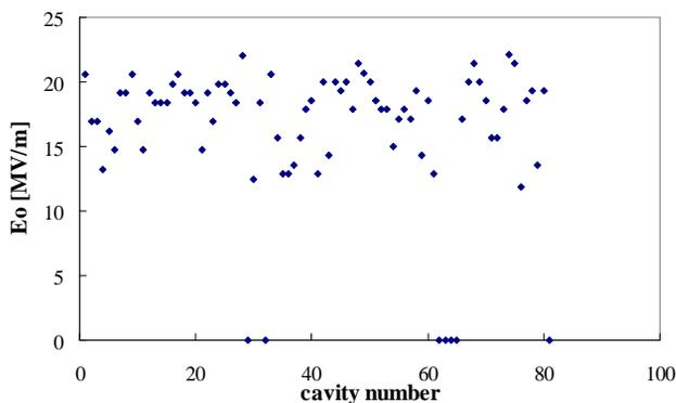
Figure 1: Plot of cavity field  $E_o$  vs. cavity number. Quite significant variation is observed besides that six cavities are off.
