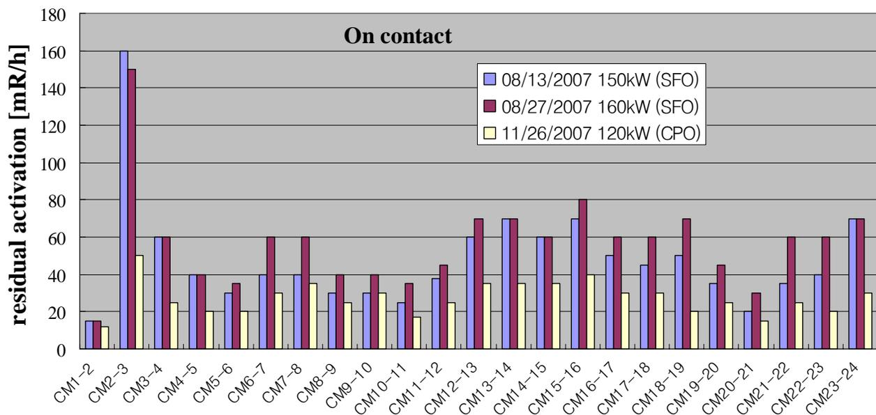
Figure 5: Plots of the residual machine activation on contact after the beam operation for four different run periods. The 150 kW (08/13/2007) run and the 160 kW (08/27/2007) run used the “Smooth Focusing Optics (SFO)”, while 120 kW (11/26/2007) run the “Constant Phase Optics (CPO)”.
