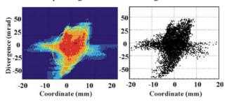
Figure 4: Measured  ${}^{12}C^{4+}$  emittance at the RFQ entrance (left) and generated particle distribution to be used for simulation.
