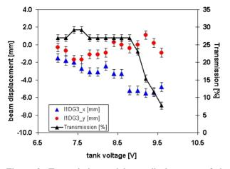
Figure 2: Transmission and beam displacement of the RFQ measured during commissioning in 2006.
