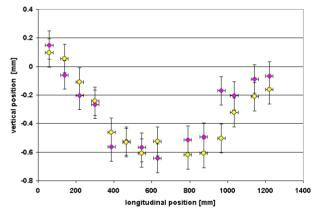
Figure 6: Vertical deformation of the CNAO RFQ electrodes measured on the upper and lower rods for a fixed (red) and loosened (yellow) tank.
