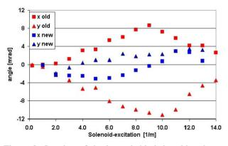
Figure 3: Steering of the beam behind the old and new Solenoids depending on their field strengths.
