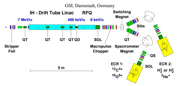
Figure 1: Layout of the Injector Linac [1]. QS = Quadrupole singulet, QT = Quadrupole triplet, SOL = solenoid, magnetic focusing and steering magnets (green), profile grids and the tantalum screen (red), and the beam current monitors (blue).
