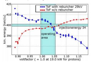
Figure 9: Measurement to adjust the rebuncher gap voltage [6].
