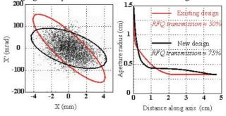
Figure 5: Dynamion simulation of the transmission improvement through the old and the new input radial matcher design using the particle distributions generated from the measured emittances (Figure 4).
