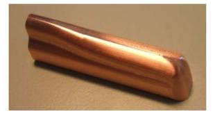
Figure 7: Final test piece of the RFQ radial matcher section to check the production procedures.
