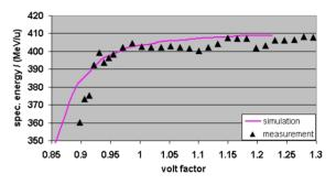
Figure 11: The RFQ energy scan with the rebuncher in the dummy position (blue) and the theory curve (red).
