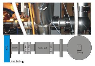
Figure 10: A photo of the diagnostics test bench as currently installed at Risø for RFQ energy measurements (top) and a schematic drawing (bottom).
