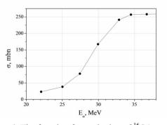
Figure 6: The function for excitation of  ${}^{16}O(\alpha, pn){}^{18}F$ .
