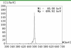
Figure 2: Output beam energy spectum.
