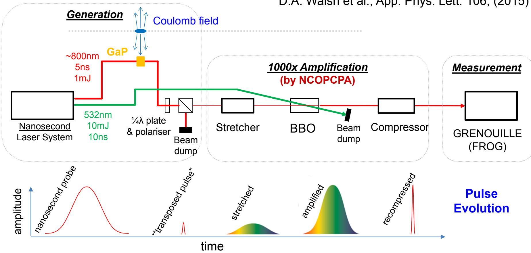
1. Nanosecond laser-derived single-frequency probe brings reliability
