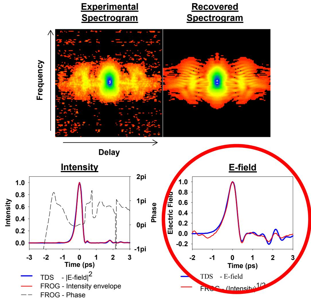
0.55 ps pulse measured with a 10 ps transform limited probe!
