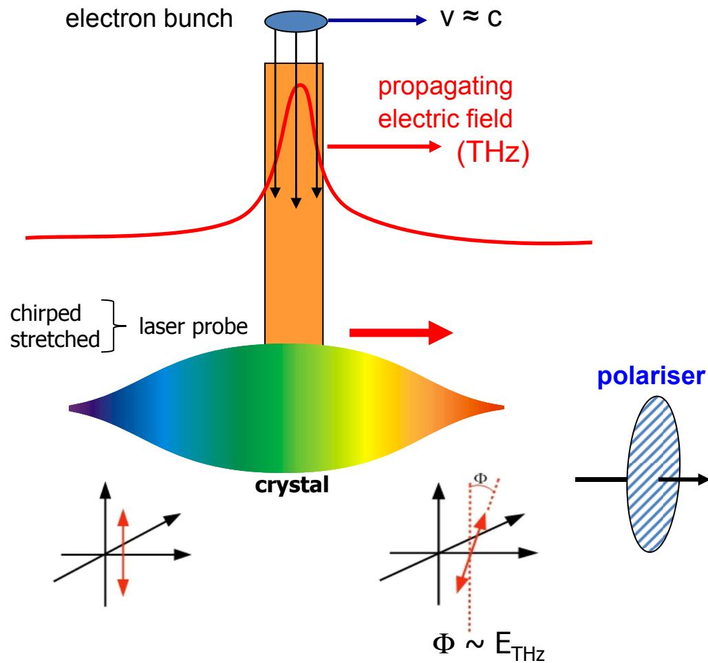
Decode: temporal intensity variations in single laser pulse via **single-shot cross correlation** in a BBO crystal
