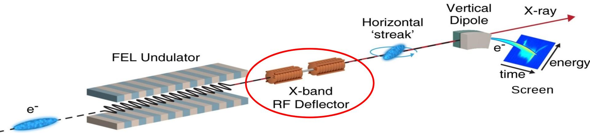
Imaging the temporal profile of the electron beam by horizontally streaking with an RF deflecting cavity and measuring the time-dependent energy via a vertical spectrometer.
