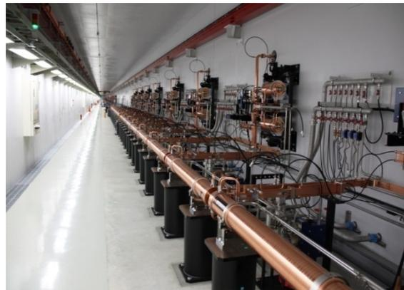
High-gradient C-band accelerator
