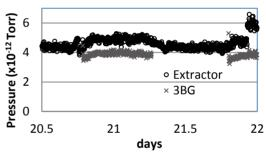
Figure 4: Study of gauge heating effect by measuring pressure in a chamber while one gauge was turned on and off. Note the time scale of days to let the system settle between state changes.
