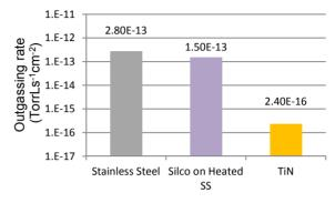
Figure 1: Best outgassing rate achieved for each chamber at room temperature of 25°C: the bare steel (304L stainless steel), the a-Si coating on 400°C heat treated steel, and the TiN coating.
