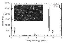
Figure 2: XPS analysis of the Ti:N coating, showing prevalence of Ti and N in the coating, and SEM image inset showing inhomogeneity in the coating.
