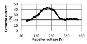
Figure 3: Measurment of the x-ray limit for an extractor gauge. The x-ray limit was measured by varying the repeller voltage on an external power supply and measuring the collector current. For increased sensitivity, the collector current was measured on an electrometer. The pressure during this measurement was in the low  $10^{-12}$  Torr range, with an x-ray limit of approximately  $1\times10^{-12}$  Torr.
