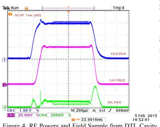
Figure 4: RF Powers and Field Sample from DTL Cavity 2 with Beam Loading, ~2.9 MW peak power.
