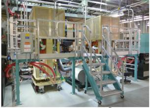
Figure 3: Dual FPAs with Diacrodes<sup>®</sup> installed.
