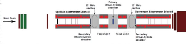
Figure 1: Final configuration of MICE cooling channel, showing two RF cavity modules.
