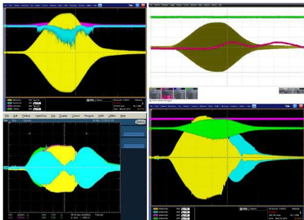
Figure 5: Scope signals during B=5 T run at ~11MV/m. Top Left: PU2, SPS upstream, SPS downstream, Light#3; Top Right: PU1, Faraday Cup, Light #1 and #2; Bot. Left: Forward and Reflected powers from Right and Left Coupler arms; Bot. Right: Forward and Reflected powers at Klystron, Light #4, NaI crystal.
