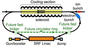
Figure 1: A schematic drawing of a bunched beam cooler based on an ERL, with bypass circulator ring connection in green.
