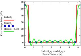
Figure 2: Ideal kicker voltage pulse (red) and bunch train scheme (blue) to kick every 10<sup>th</sup> bunch, and the reconstructed kicker pulse with the first 10 harmonic modes (green).
