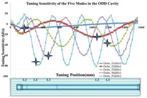
Figure 7: Tuner position simulation for the 5 harmonic modes cavity with a small cylinder perturbation.
