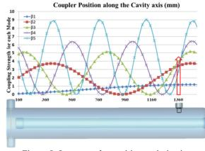
Figure 8: Loop coupler position optimization.
