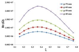
Figure 5: Optimization of the inner conductor for two different gaps when b is 157 mm.
