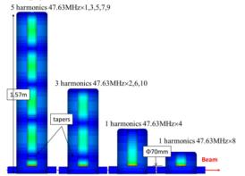
Figure 6: Harmonic modes in four cavity system with the highest harmonic electric field distribution shown in each cavity.
