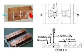
Figure 2: Sketch of W-band wakefield structure.
