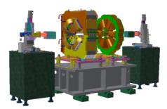
Figure 4: Vibrating wire alignment system model.
