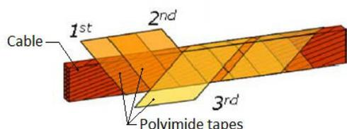
Figure 2: Superconducting cable insulation.
