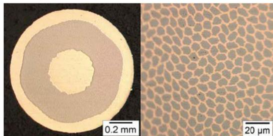
Figure 1: Transverse cross section of composite NbTi/Cu wire.
