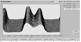
Figure 8: Tomoscope view of accelerated beam. MA cavity providing h=1 component (780E10ppb).
