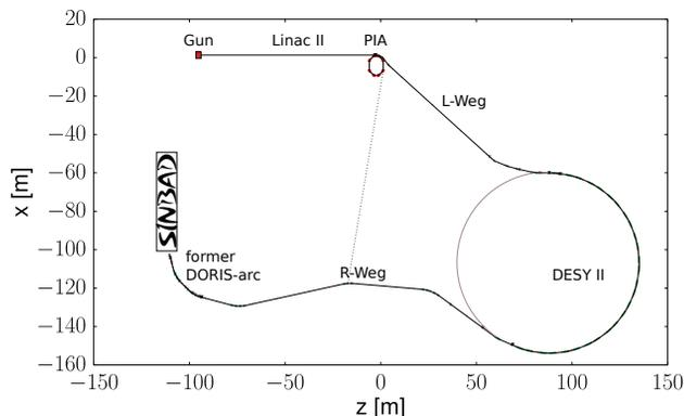
Figure 1: The geometric layout of the beam transport system from the electron gun of Linac II up to the SINBAD facility.
