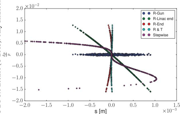
Figure 5: The longitudinal phase space distribution at the photo-cathode, the exit of the Linac II and at the end of the transfer line. For the transfer line three different models (single element with R56, single element with R56 & T566, element wise tracking with second order transfer matrices) were used. It shows that higher order terms are dominating the bunch length.
