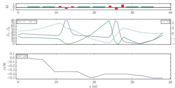
Figure 4: The proposed beam line layout and the corresponding beam optics of the final arc.
