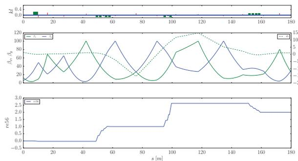
Figure 3: The proposed beam line layout and the corresponding beam optics of the "R-Weg".
