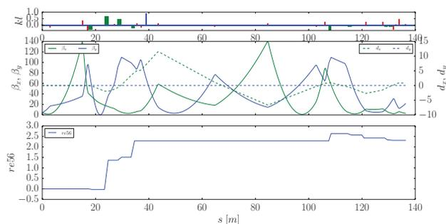
Figure 2: Possible beam-optics solution for a bypass around PIA and the subsequent transfer line to the start of the DESY synchrotron.
