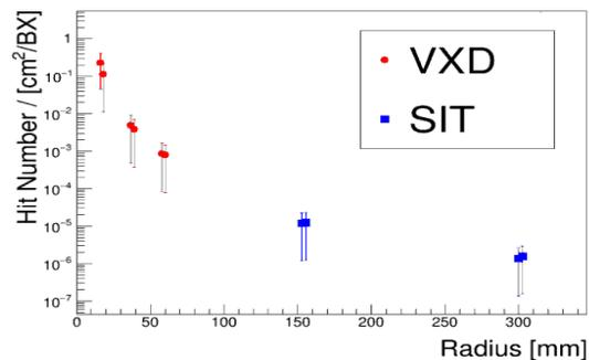
Figure 4: The hit number of The incoherent  $e^+e^-$  pair in the inner detectors.
