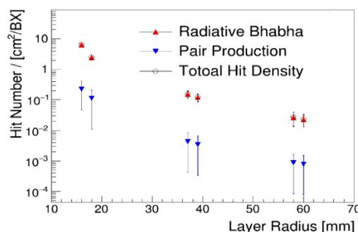
Figure 7: The hit number of Radiative bhabha scattering in the inner detectors.
