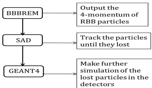
Figure 5: the process of the simulation on radiative Bhabha scattering.
