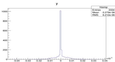
Figure 8: The vertical r.m.s BPM readings after orbit correction.
