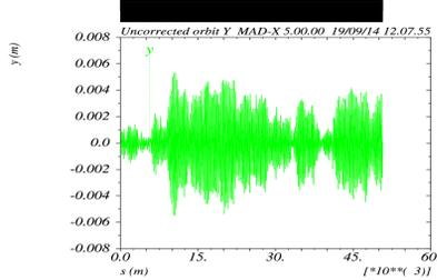
Figure 2: Vertical orbit deviation before correction.
