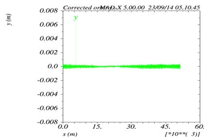
Figure 6: The vertical orbit after orbit correction.
