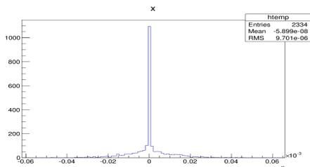
Figure 7: The horizontal r.m.s BPM readings after orbit correction.
