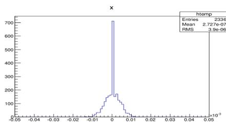
Figure 9: The horizontal correctors' statistic after orbit correction.
