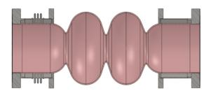
Figure 1: 1500 MHz cavity geometry.
